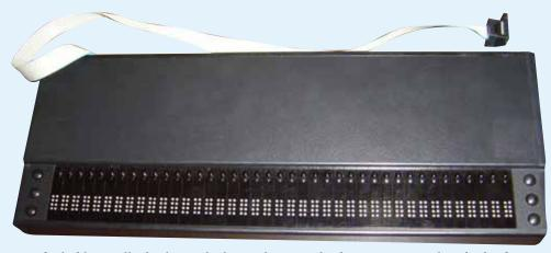
Refreshable Braille displays, which attach to standard computers, use hundreds of tiny electronic pins that move up and down to convert computer text into Braille. CSB's software converts Torah CDs into the refreshable Braille format, giving observant blind users instant access to over 500 Torah works including the Talmud, Midrash and even obscure halachic works.
